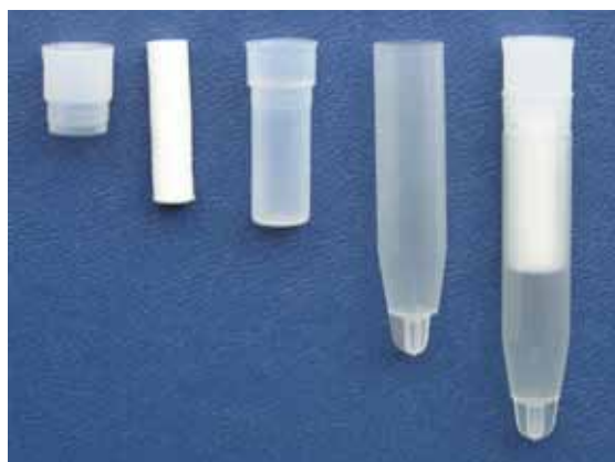
Fig. 1 Photograph shows the Salivette device for the collection of saliva; from left to right: stopper, cotton swab, cotton swab holder with a hole at the bottom, collection tube and the complete device.
