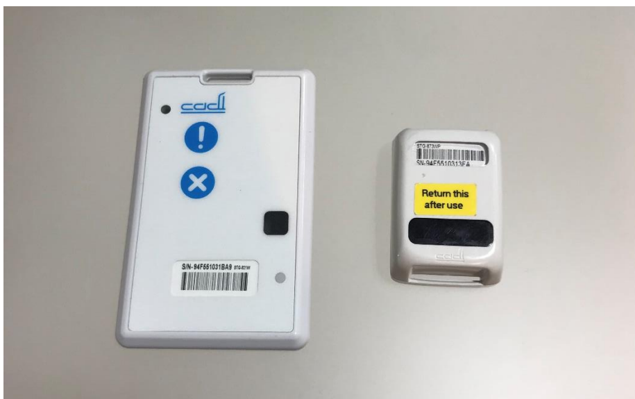
Fig. 1 Photograph shows the real-time location system tag (left) carried by staff when working in the emergency department and the tag attached to an identification band on a patient's wrist (right).
