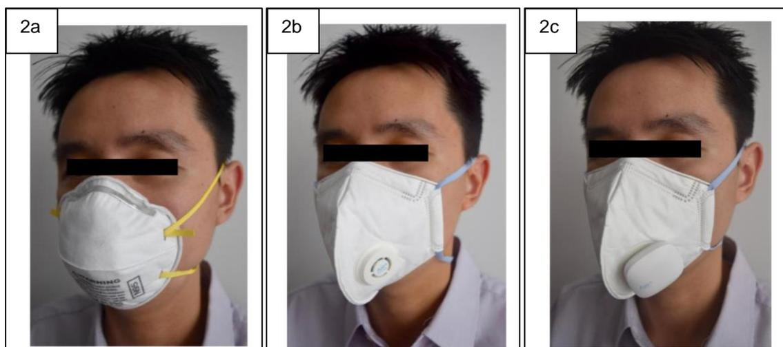
**Fig. 2** Photographs show personnel wearing (a) standard FFR; (b) FFR with EV; and (c) FFR with EV+AVS. The FFRs were the National Institute for Occupational Safety and Health-approved N95 particulate FFRs. Respirators were self-checked to determine good fit prior to usage according to manufacturer's instructions. AVS: active venting system; EV: exhalation valve; FFR: filtering facepiece respirator
